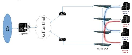
**Surveillance Applications**: CCTV cameras can be powered on & backhauled using Power over Ethernet ONTs on a single fiber.
