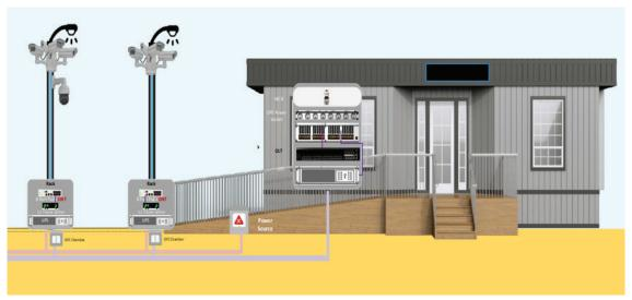
**Wi-Fi Internet**: Wi-Fi Access Points can be powered on & backhauled using Power over Ethernet ONTs to cater to internet to citizens at various Hot-spots.
